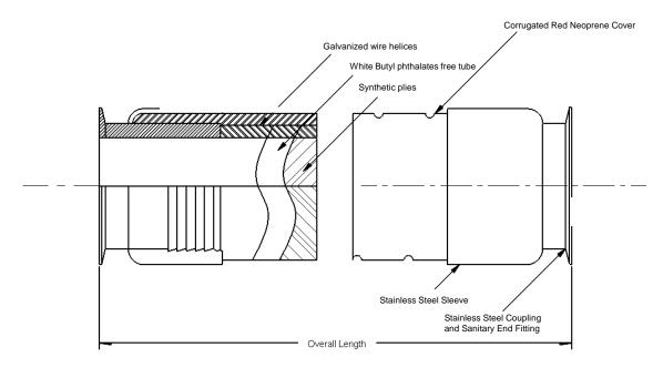
Available with clamp type, bevel seat and nut, cam lock, flanged, threaded or weld ends in T304 or T316 stainless steel.
