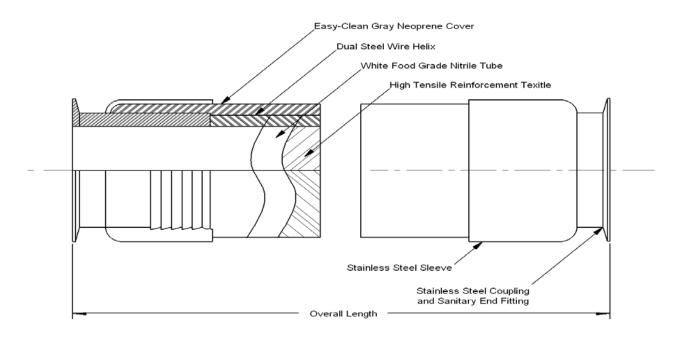
Available with clamp type, bevel seat and nut, cam lock, flanged, threaded or weld ends in T304 or T316 stainless steel.
