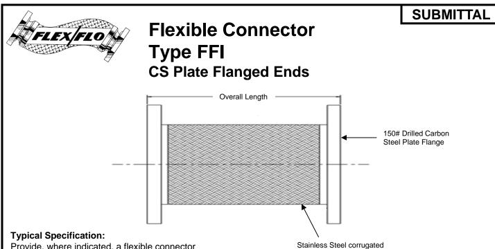
Provide, where indicated, a flexible connector consisting of 300 Series stainless steel corrugated hose surrounded and supported by 300 Series stainless steel braid. End fittings are to be carbon steel 150# drilled plate flanged ends. Connector to be \_\_\_\_\_ inches nominal pipe size by \_\_\_\_\_ Inches overall length; **Thermo Tech model FFI or equal**.
