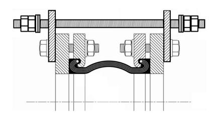
Field installed control rods perfom the same as factory installed control rods but are ideal for in-place units, unexpected system requirements, or additional number of control rods needed.
