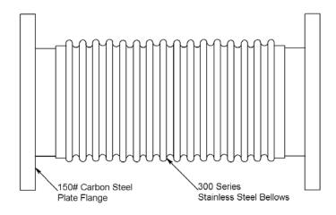
THIS VERSATILE EXPANSION JOINT WILL COMPENSATE FOR THERMAL EXPANSION AND CONTRACTION IN PIPING SYSTEMS. THE FLEXIBLE STAINLESS STEEL BELLOWS EXTENDS AND COMPRESSES WITHOUT THE USE OF SHORT-LIVED SLIP JOINTS, "O" RINGS, OR EQUALIZERS, TO GIVE MAXIMUM DEPENDABLE SERVICE.
