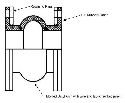
These connectors are furnished complete with flange retaining rings and control rod sets.
